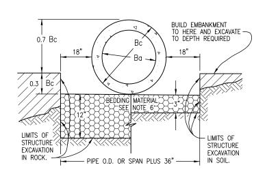
NOTE: BC IS THE OUTSIDE DIMENSION FOR DIAMETER, SPAN OR RISE.
